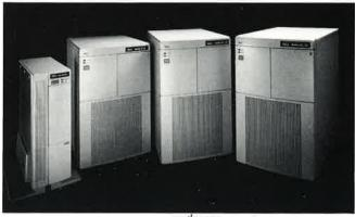
The XL family is MC68020-based, with up to 16MB main memory, up to 2GB of disk storage and can accommodate up to 32 users. Plus, it runs a range of IBM and other communications protocols and offers advanced networking capabilities.
