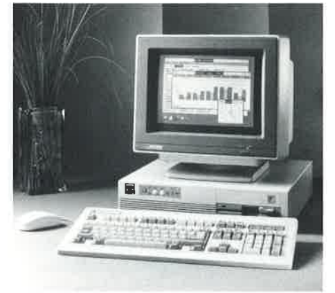
The Prize 16 MHz 386sx system with 1 MB memory, 30 MB hard disk, 14" color VGA monitor, VGA card, 5 1/4" floppy drive, 101 Keyboard, MS DOS 3.3, Microsoft Windows 3.0, and a Microsoft Windows 400 DPI serial mouse.
