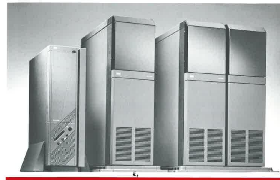
The Series 5000i Model 510 and Series 9000i Model 920 are the first in a new family of Wyse-designed UNIX systems that can support from two to 128 active users, with connectivity of up to 288 serial devices.
