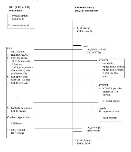
The following diagram shows the execution flow for the FUNCTION/PROCEDURE (interface):
